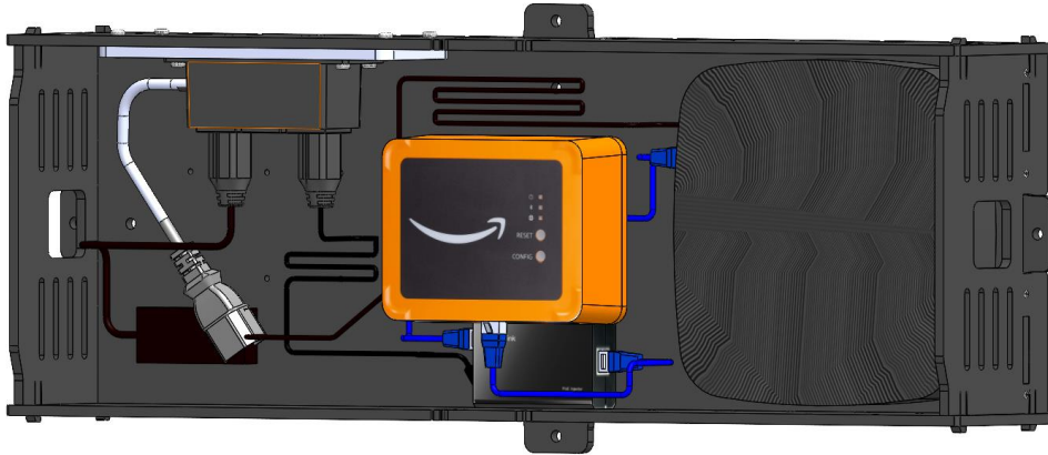
Figure 6. Proposed connections and cables path
